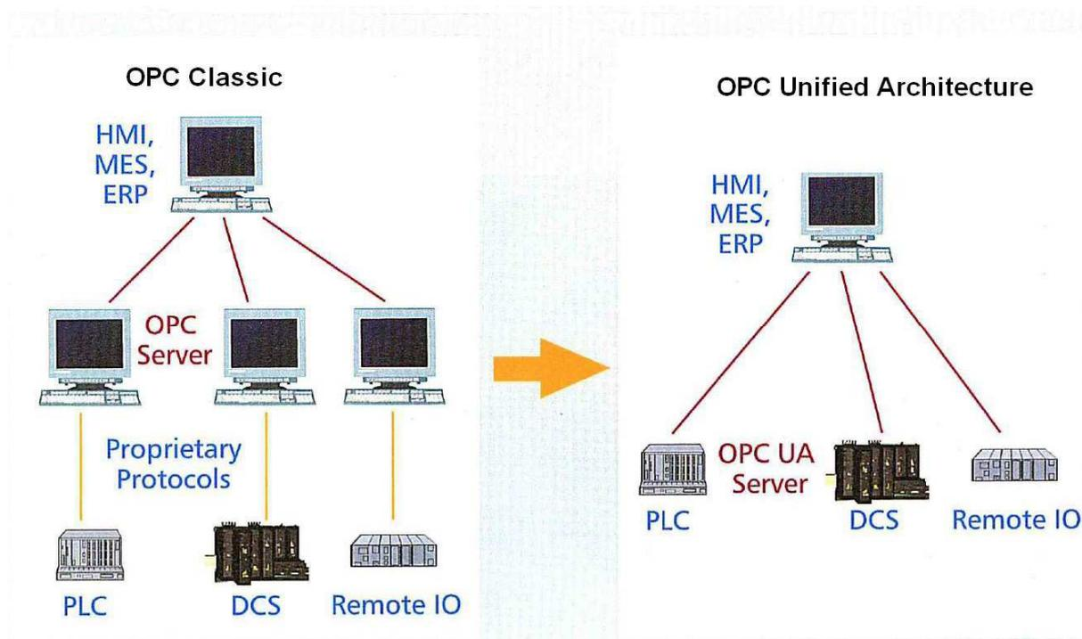
Fig. 1: OPC UA architecture: OPC UA allows the implementation of servers in embedded systems, thus opening the door to new automation concepts.
