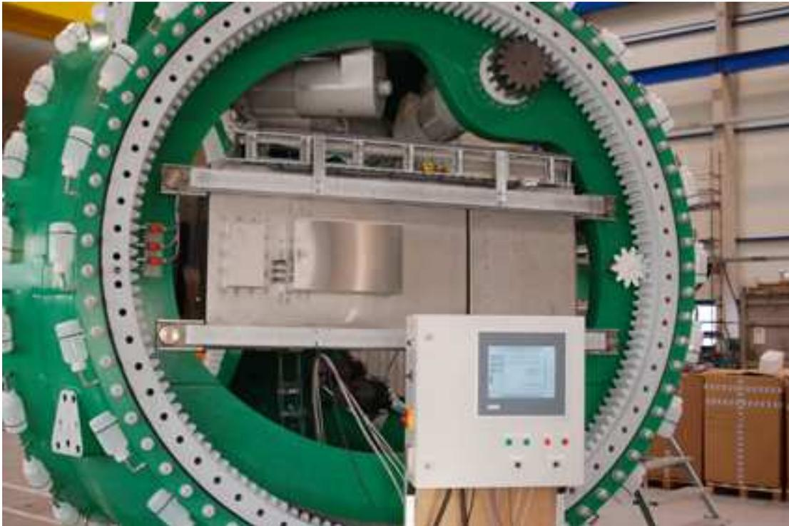
Fig. 3: Areva: The rotor of the AREVA wind turbine features a controller with an OPC UA server. This provides the basis for communication between the turbine and the central operating station on the mainland.
