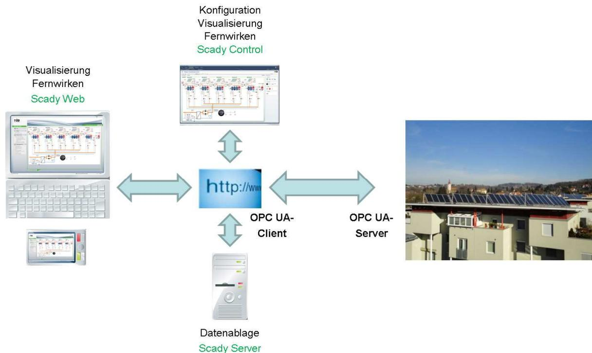
Fig. 2: In a large residential complex in Graz, Austria, the operation and monitoring functionalities have been implemented for the entire local heating grid of several buildings, for the heating system for 59 residential units, and for a 300 sq.m solar thermal system.
