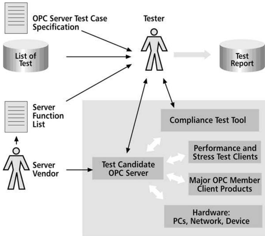
Fig. 1 – OPC Server test environment
